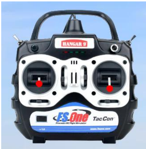
Figure 3. Right control stick pulled back—plane pitches up.
