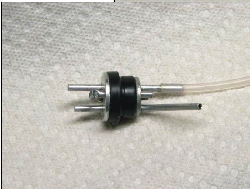
Left: Fuel stopper with short piece of aluminum tubing inserted. Tubing end is crimped with pliers.
