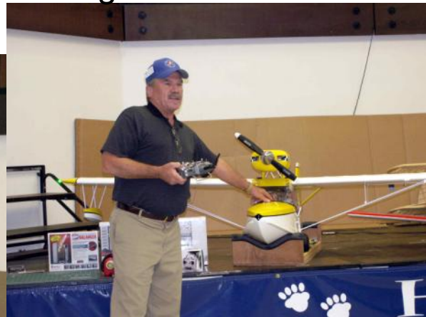
Above: Don Coulter and his scratch built Kingfisher. Retracts rotate forward and up. Deployable water rudder. Yet to fly.
