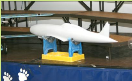
Babe Caltabiano describes his plug construction technique, aka lots of Bondo. Plug is very heavy.
