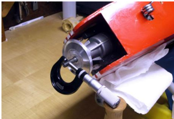
Left: Micrometer used to check propeller drive shaft diameter. In this case it measured 0.313 inch.
