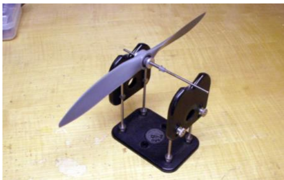
Left: Finished product. Prop balances level when sufficiently balanced.
