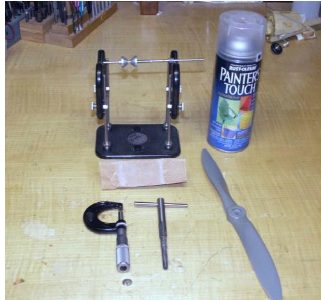
Left: Micrometer used to check propeller drive shaft diameter. In this case it measured 0.313 inch.
