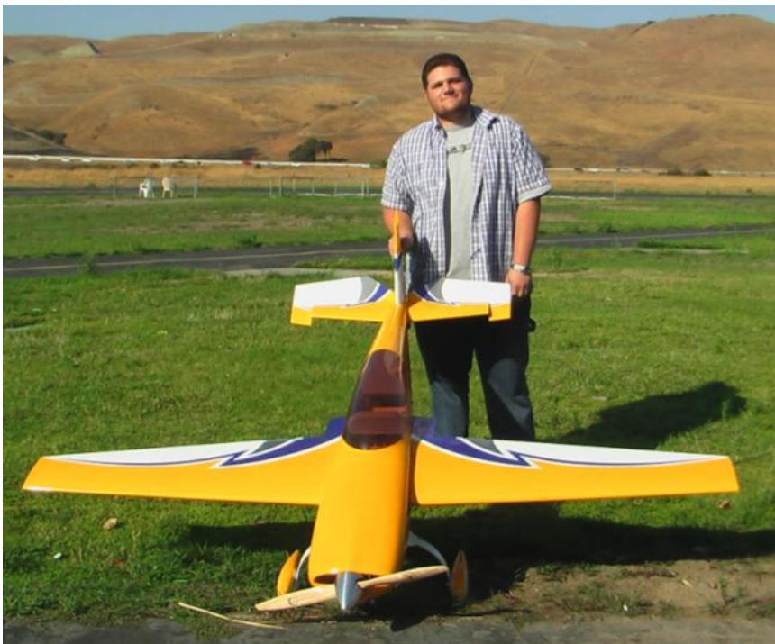
Sean Sorkhabi with his Aero Works 30% Extra 300 with a DLE-55, Hitec servos, guided by a Futaba 12FG 2.4 GHz. Sean's uncle Jay took the photo.
