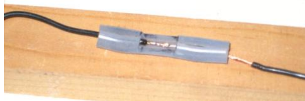
Photo 3: The glow tubing is centered on the block with nails. The nails are hammered down into the tubing.
