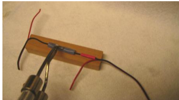
Photo 5: Let the soldering begin. Notice shrink tubing on the right side ready to be slid over the solder joint. The Soldering Jig holds the wire to be soldered in place.
