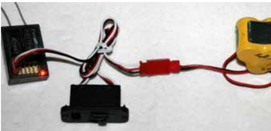
My experience measuring battery current to detect a stalled servo.
