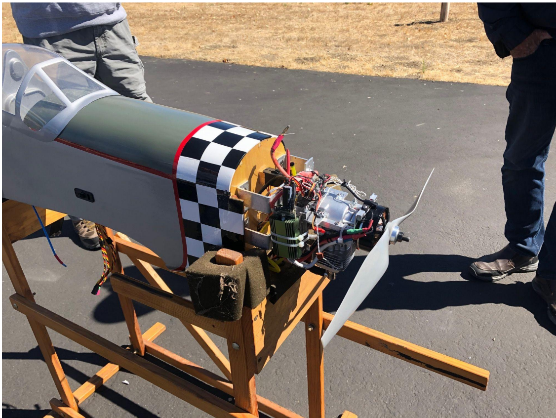
Mike Leggett's newest engineering feat - a hybrid gas/electric power plant for his Mustang.
