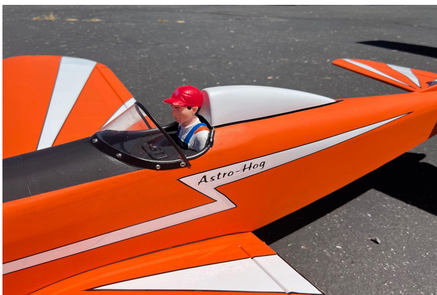
Above and Below: Bob Zuk's SIG Astro-Hog. Covered with Oratex fabric, with O.S. 2 stroke gasoline engine
