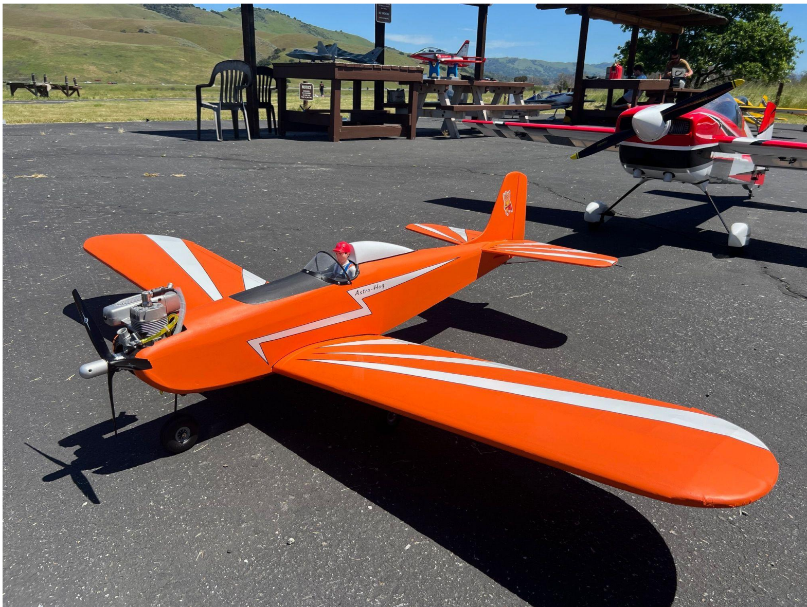
Above and Below: Bob Zuk's SIG Astro-Hog. Covered with Oratex fabric, with O.S. 2 stroke gasoline engine
