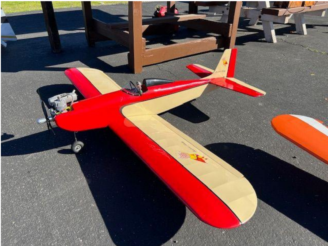
Above and Below: Bob Zuk's SIG Astro-Hogs. Covered with Oratex fabric, with O.S. 2 stroke gasoline engines
