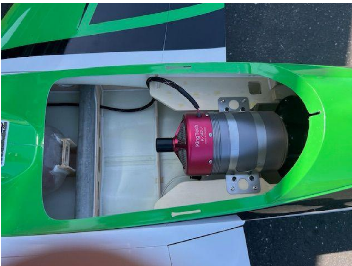
Above and Below: SCCMAS Member Alex Saroyan's CARF Rebel Classic, with Kingtech K-142 Turbine Engine for power.
