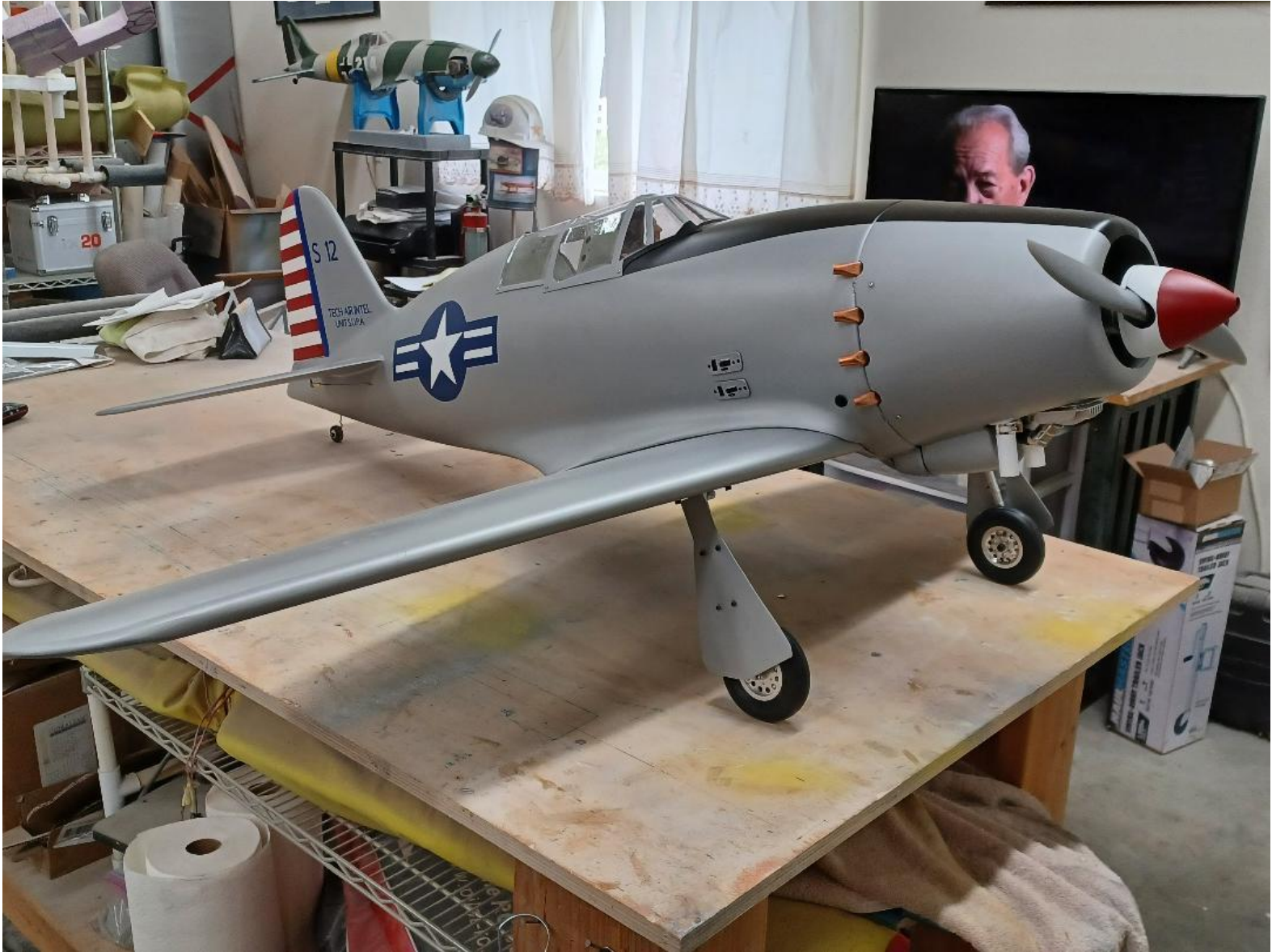
Above and Below Right: Babe Caltabiano's scratch built Japanese Raiden. Babe's version is a captured Raiden, with a wingspan of 63 inches; weight 14 lbs; engine DLE20. Fiberglass fuselage and foam wing covered with balsa and fiberglass, etc.
