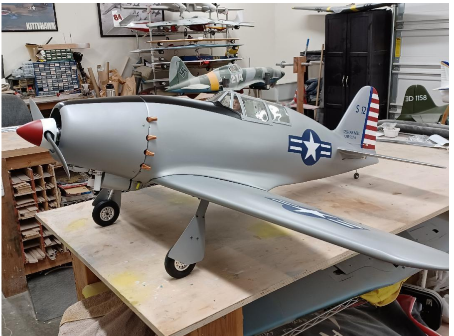
Above and Below Right: Babe Caltabiano's scratch built Japanese Raiden. Babe's version is a captured Raiden, with a wingspan of 63 inches; weight 14 lbs; engine DLE20. Fiberglass fuselage and foam wing covered with balsa and fiberglass, etc.
