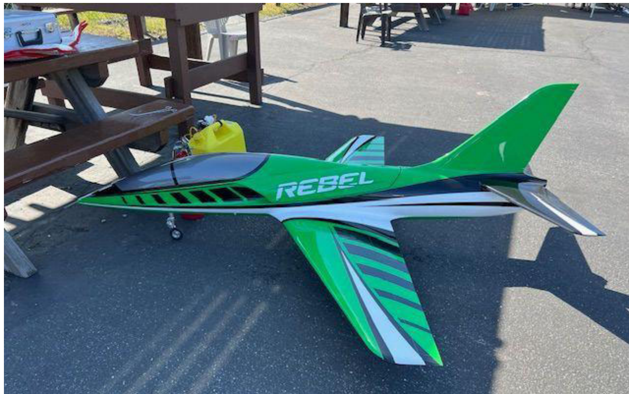
Above and Below: SCCMAS Member Alex Saroyan's CARF Rebel Classic, with Kingtech K-142 Turbine Engine for power.
